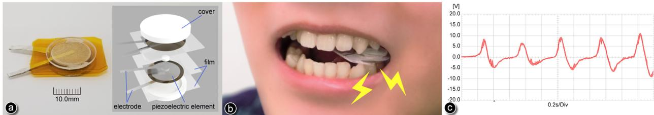
Figure 1. (a) Electric taste apparatus: Unlimited Electric Gum. (b) Image of a user chewing the apparatus. (c) Waveform of the piezoelectric voltage.
