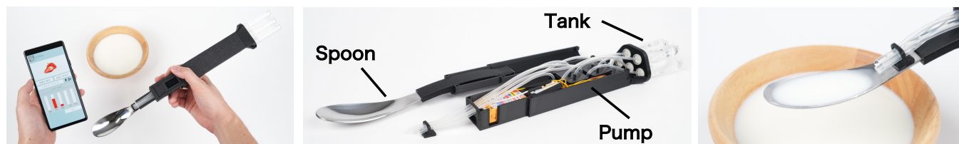
Figure 1: (Left) Our proposed hardware and software. (Center) The hardware is equipped with five tanks, five pumps, and one M5StickC Plus 2. (Right) The system can produce a variety of tastes by mixing five basic taste solutions in each bite.
