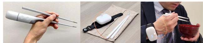
Figure 2: Initial design of integrated chopstick (left). Revised design with smartwatch structure (center). User eating miso soup with chopstick.
