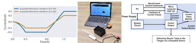
Figure 1: Stimulation waveform (left), experimental setup (center), and current output device configuration (right) in [8].
